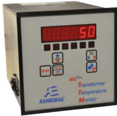
144 x 144 DIN Panel Mounted Version 144mm (W) x 144mm (H) x 220mm (D) Cutout: 138mm x 138mm + 0.5/-0.00
