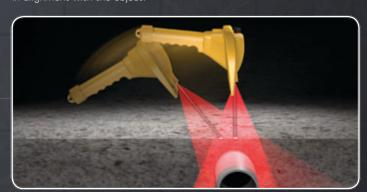
Pivot the AML until it is perpendicular to the ground, and directly above the target. You can now scan the ground in parallel for the entire length of the object, marking its location and run direction as you track it.
