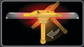
While the left or right target indicator is activated, rotate the AML until it becomes parallel with the subsurface object. Both the left and right LED target indicators will light simultaneously when the unit is in parallel and in alignment with the object.
