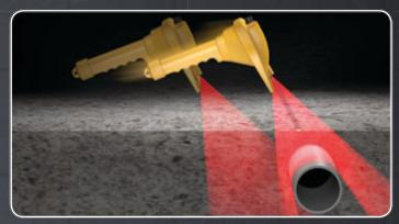
First, sweep the area of interest in a back and forth "W" action, completely scanning the area for buried objects. The left or right target indicator will activate, with an audio tone and laser marker, when an object is detected
